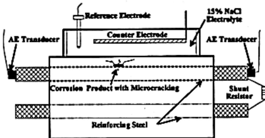
**FIGURE 1 - Schematic of Rebar Test Specimen**
