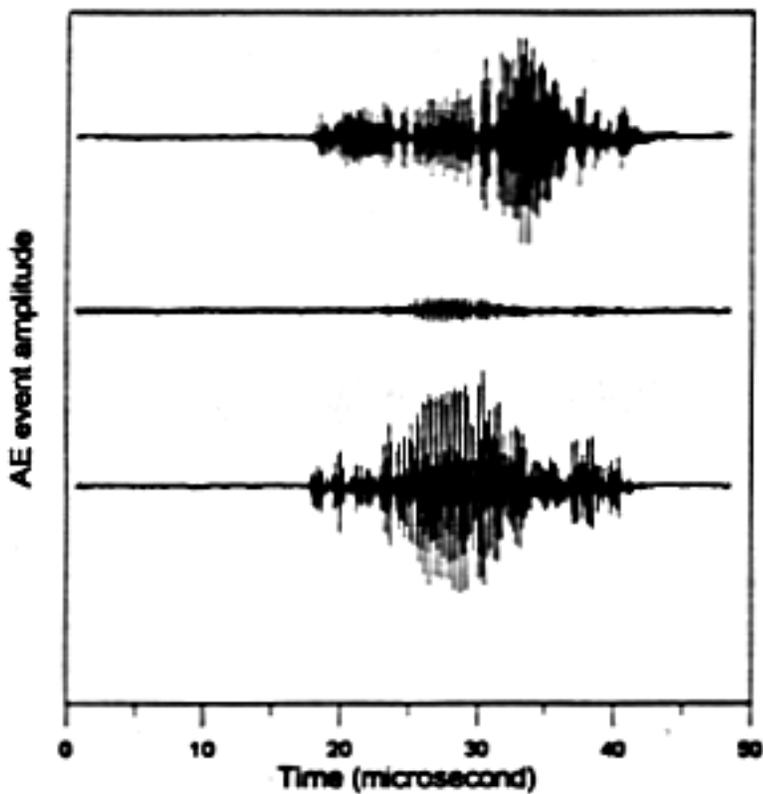
**FIGURE 3b - AE Signal at the Three Transducers for a Single AE Event**
