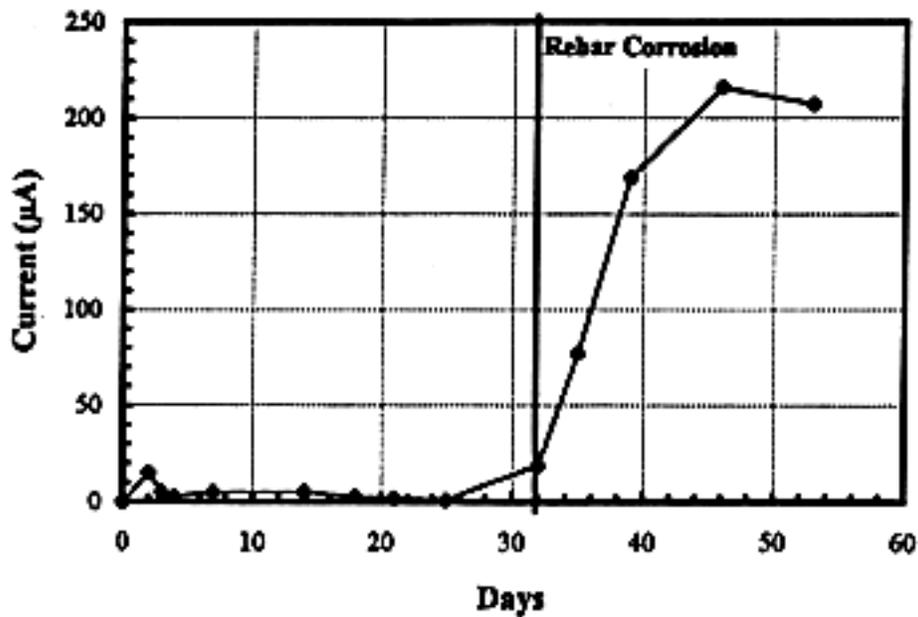
**FIGURE 4a - Galvanic Current versus Exposure Time**
