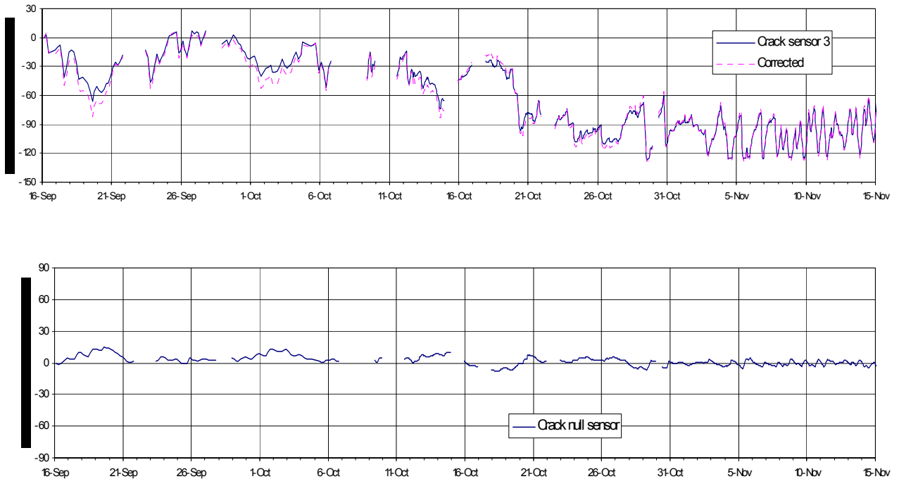
Figure 6: Crack 3 Response Corrected for Null Response Showing Relatively Small Effect of the Null Response
