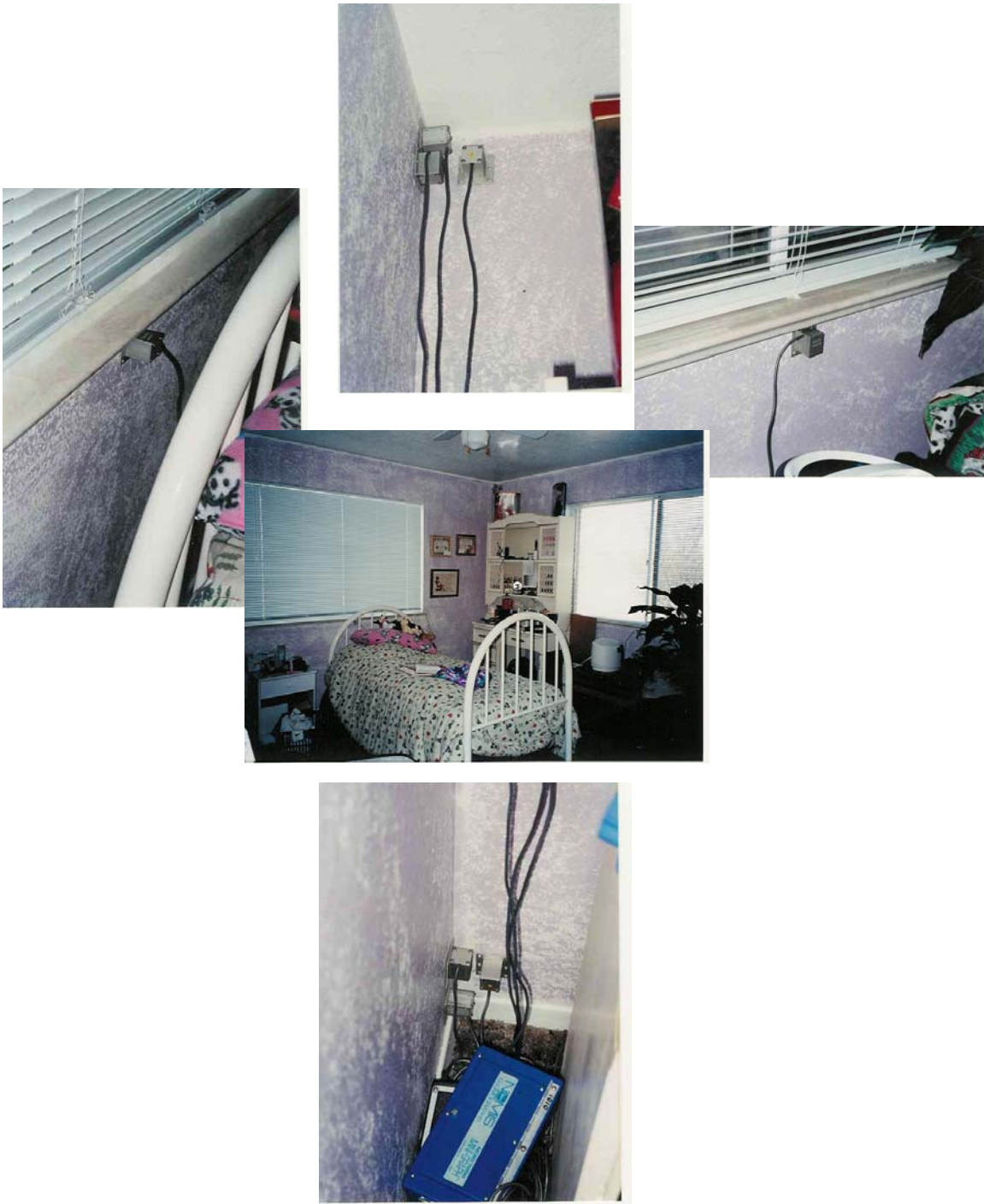
Figure 2 Photographs of Transducer Locations for Measurement of Structural Response Showing Individual Midwall transducers (left and right) as well as corner clusters (top and Bottom)
